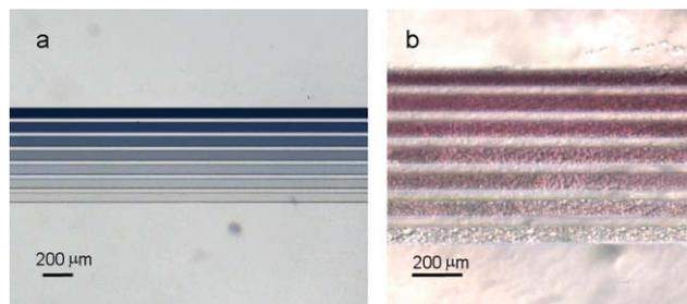
**Fig. 5** Microfluidic arrays with upstream microfluidic mixers. To lower the number of independent inlets into the device, micromixers can be incorporated upstream from the microchannel arrays: (a) represents experiments in which a concentration gradient was generated in an array of channels, and (b) is a monolayer of NIH-3T3 cells immobilized in such a microfluidic array.
